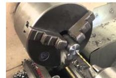
**Centre Drilling:** Drilling a hole in centre of the workpiece
